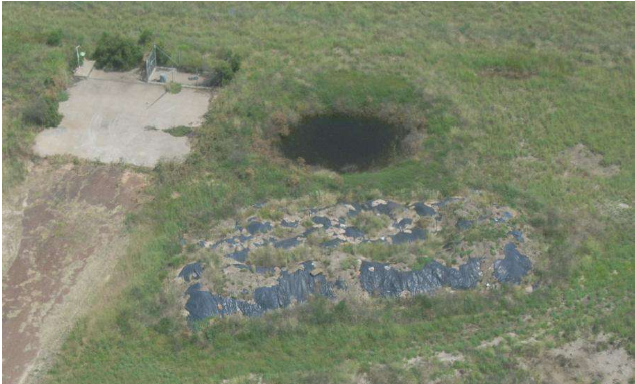
Plate 5 – Contaminated soil stockpile covered with plastic & soil, December 2010.
