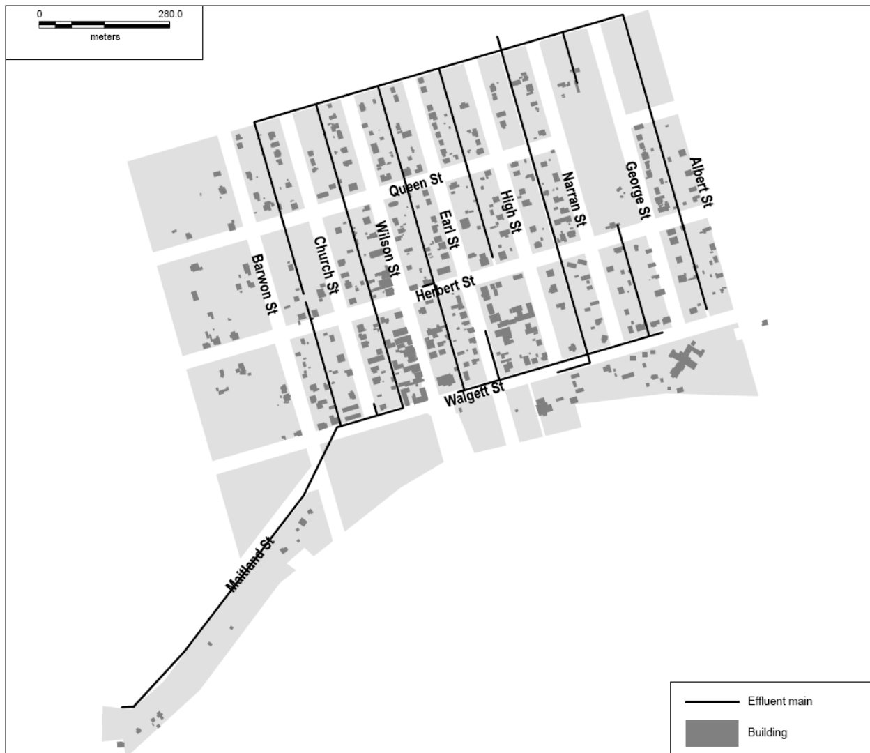
Figure 1 – Extent of urban development and effluent mains in Collarenebri
